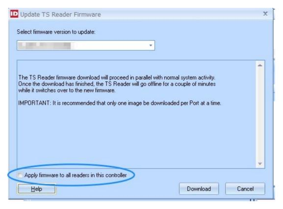
Avoid initiating parallel download of reader firmware connected under both master and downstream controllers at a time.
