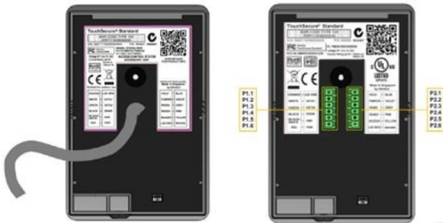
Exhibit 5: Pigtail Connector (below left) and Terminal Connection (below right)
