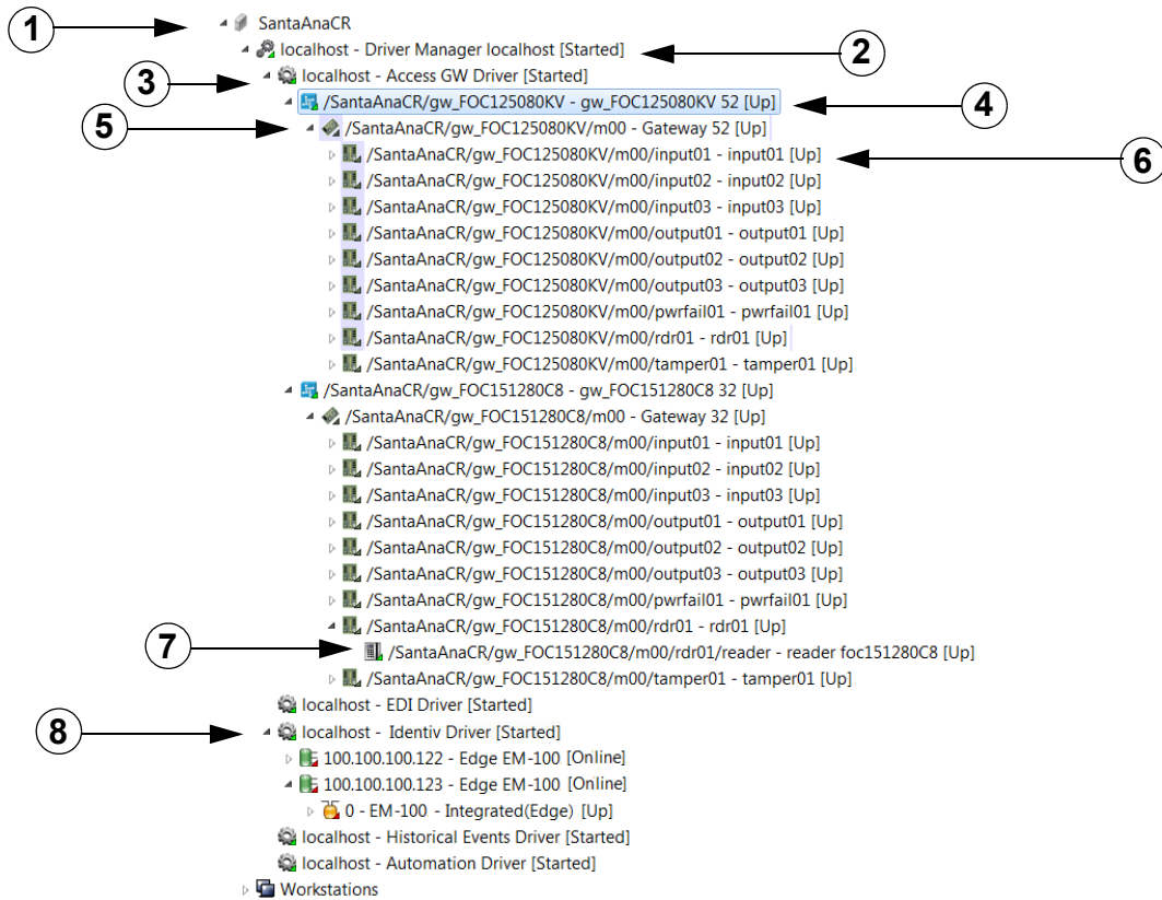
Figure 5-1 Expanded Hardware Tree: Controllers and Related Devices
