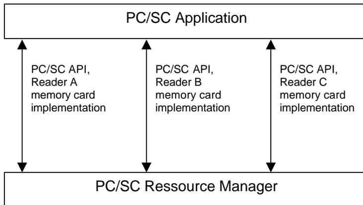
The MCard API is placed in between the PC/SC application and the Resource Manager. The application can still use all available PC/SC functionality to get the device information or monitor the card state. However, for all memory card related functionality it uses the MCard APIs.
