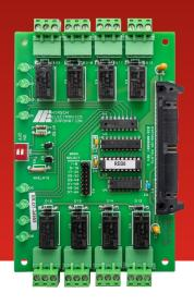
Hirsch's Relay Expansion Board (REB8) provides eight (8) additional two (2) AMP form C dry relay outputs, rated for 24VDC. These relays are socketed and removable.
