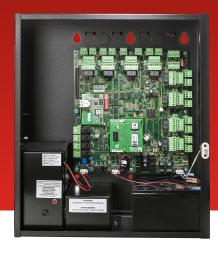
This kit replaces the previous Mx-8-N3-FICAM kit and provides the required SNIB3 built onboard, which frees up one expansion slot.
