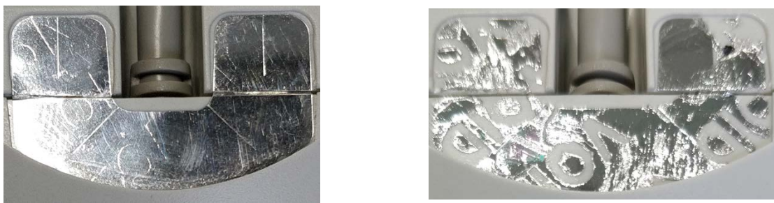
fig. seal on bottom of the SPR332 v2 left – normal seal; right – tampered seal
