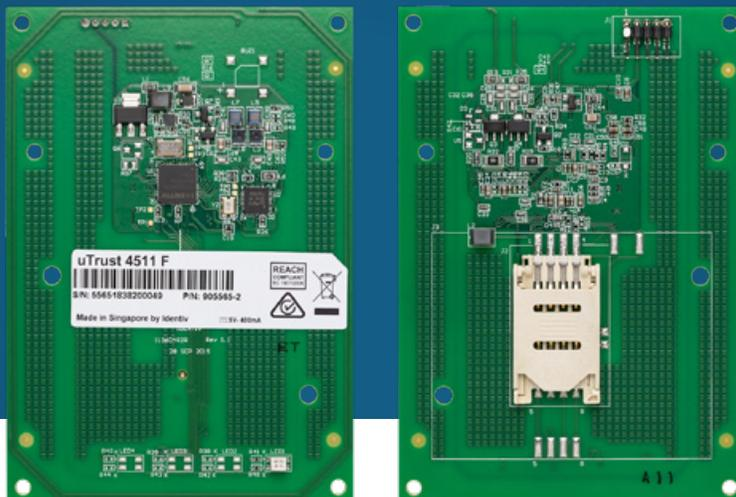
Contactless 13.56 MHz, USB-CCID, ISO/IEC 14443, and NFC module features ISO/IEC 7816 SAM support.
