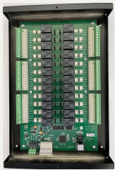
Primis Relay Encryption Bridge - Elevator Control
