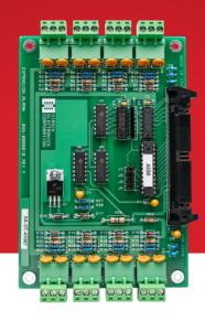
Identiv's Alarm Expansion Board (AEB8) expands the line module input capacity of a controller. AEB8 provides an additional eight (8) line module inputs per board.
